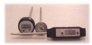
A probe thermometer is used to take food temperatures and can either be a dial or digital thermometer. Both are reliable; however, digital themometers can take temperatures of thin food while dial thermometers may have to be immersed up to 2 inches into the food to take a proper temperature.
