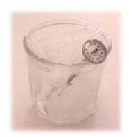
How to you know a thermometer is accurate? The answer is to check it in ice water. Water freezes at 32° F.; therefore, a glass of ice water will be very close to 32°F. By setting the thermometer in the ice water for a few minutes, you can find out if the thermometer is accurate if it correctly reads 32°F.
